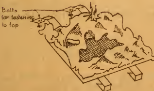
FIG 38 PORTABLE ARMORED OBSERVATION POST
